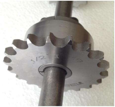
20 OR 21,22,23 ... TEETH BIG CHAIN WHEEL FOR DRIVING SHAFT (Depend on Determine the Gear Ratio & Mobile Speed)
